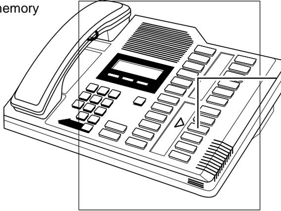
Memory buttons are the buttons with indicators other than line or Handsfree buttons. Memory buttons store telephone numbers or feature codes to give you one touch dialing or feature activation. You can change what a memory button does by just programming it with a new number or feature.
