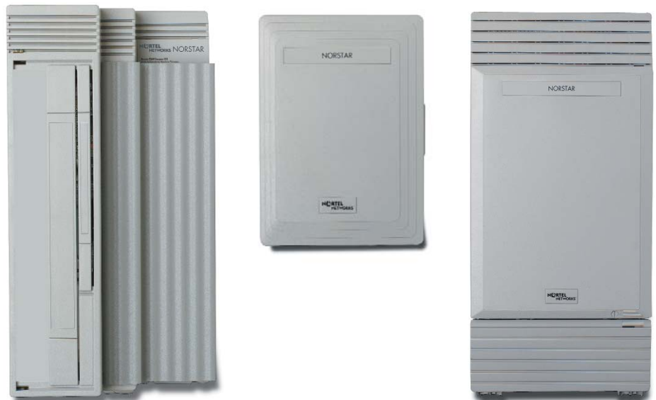
Figure 1: Norstar Integrated Communications Systems offer practical solutions. Models from left to right are the Norstar Compact ICS, Norstar 3x8 and the Norstar Modular ICS.
